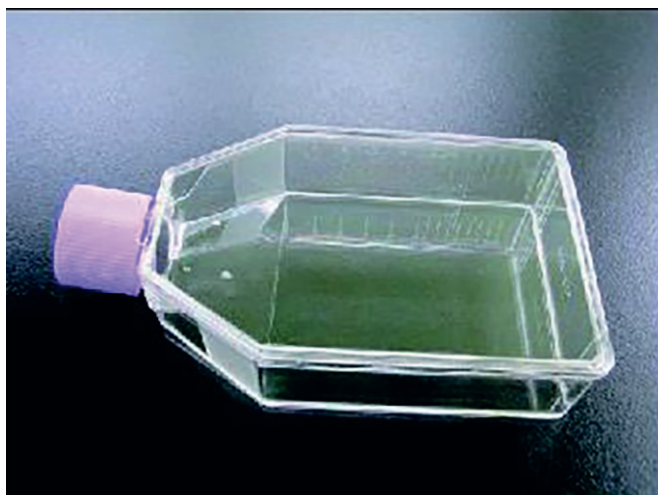
Figure 3 — Flask for cell culture use
